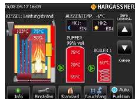
Boiler in Part-Load: Boiler is only working with half-power. Boiler and Accumulator are loaded already. Heating Circuits ensure required temperature in each living-area.
