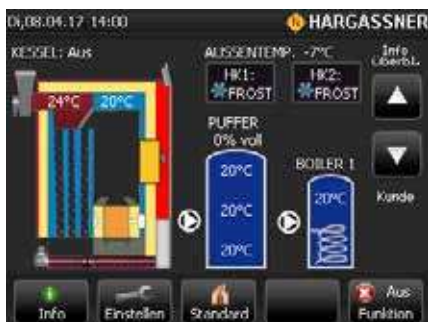
Boiler before starting: Display of Lambda Touchtronic shows a not-heated boiler. HWT and Accumulator are cold - not loaded
